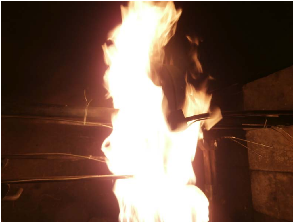
Test Gasket During Burn
