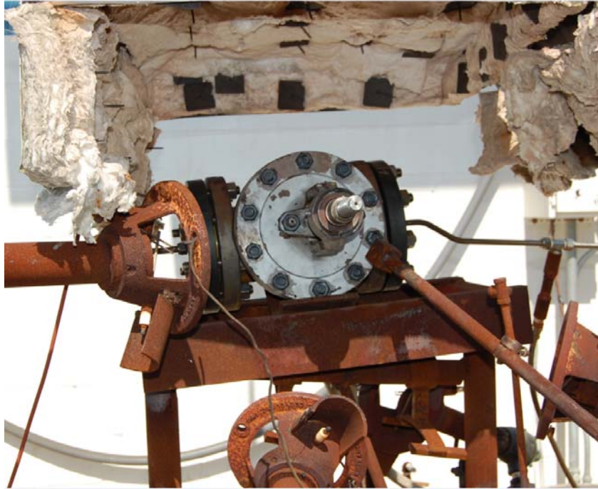
Valve in test stand prior to burn
