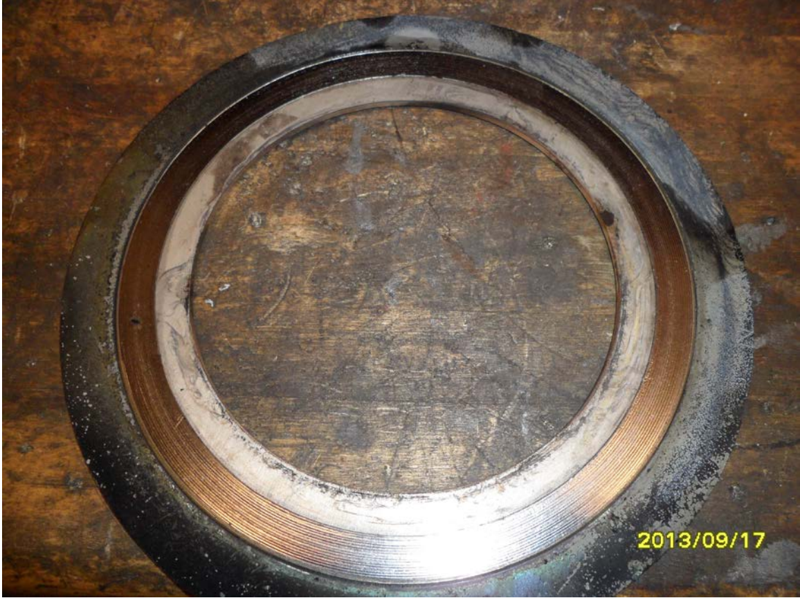
Test Gasket Post-Burn
