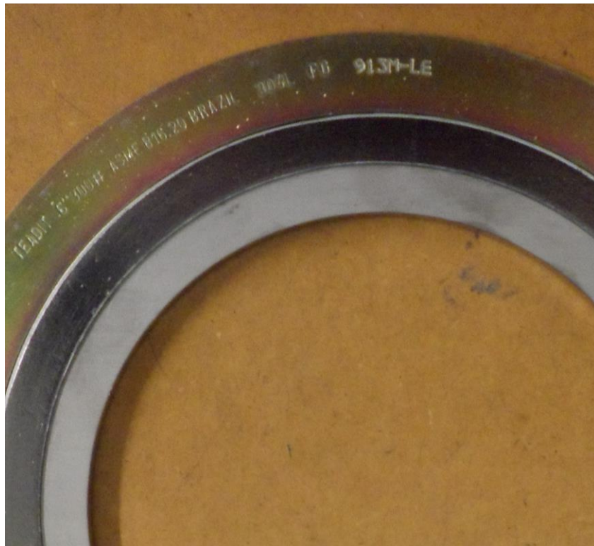
Test Gasket Prior to Burn
